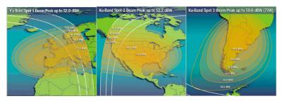
The global, hemispheric and zone beams use C-band frequencies. The spot beams use Ku-band frequencies.
